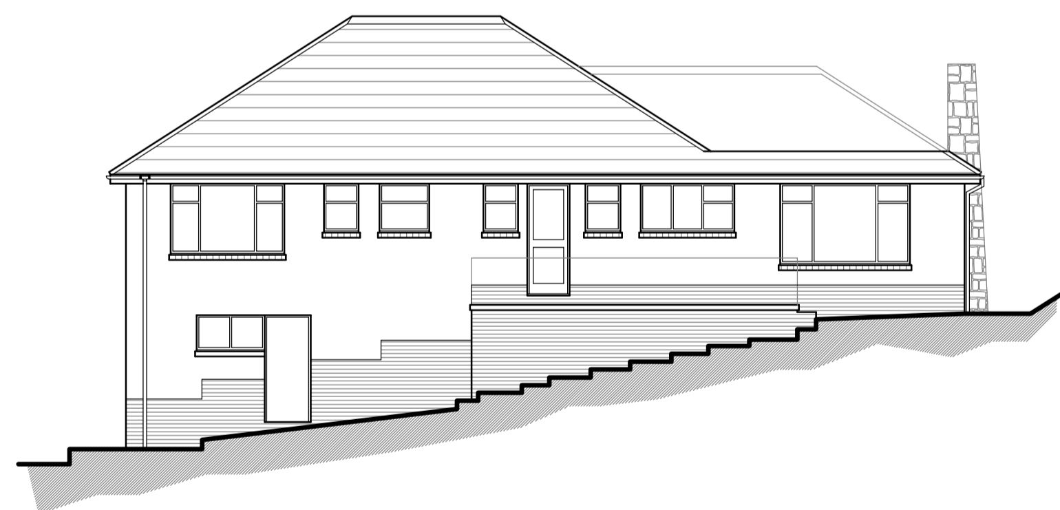
EXISTING REAR ELEVATION (north) 1:100
