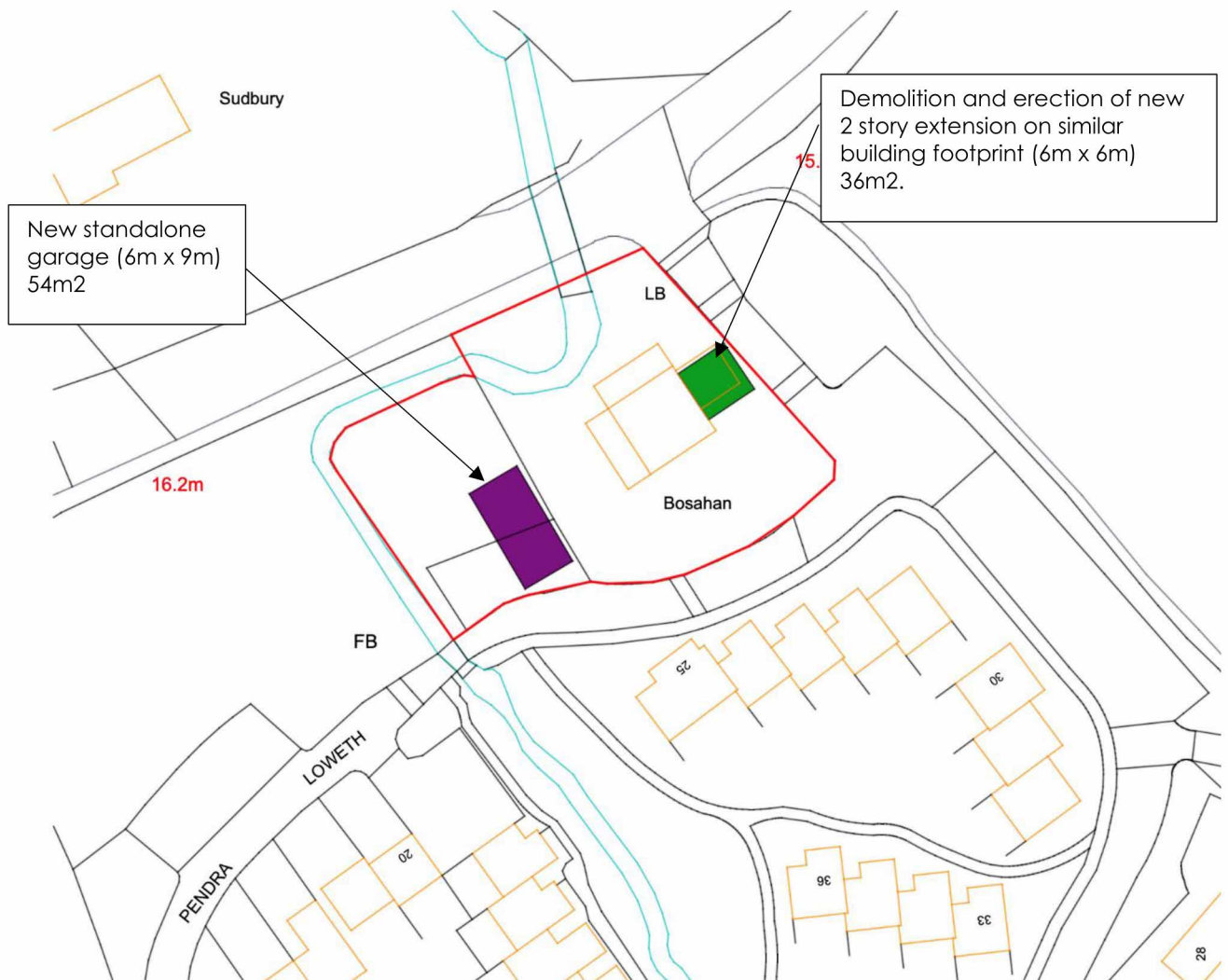
Figure 2 – Proposed Layout of the extension in green (original footprint shown in yellow) and stand alone garage
