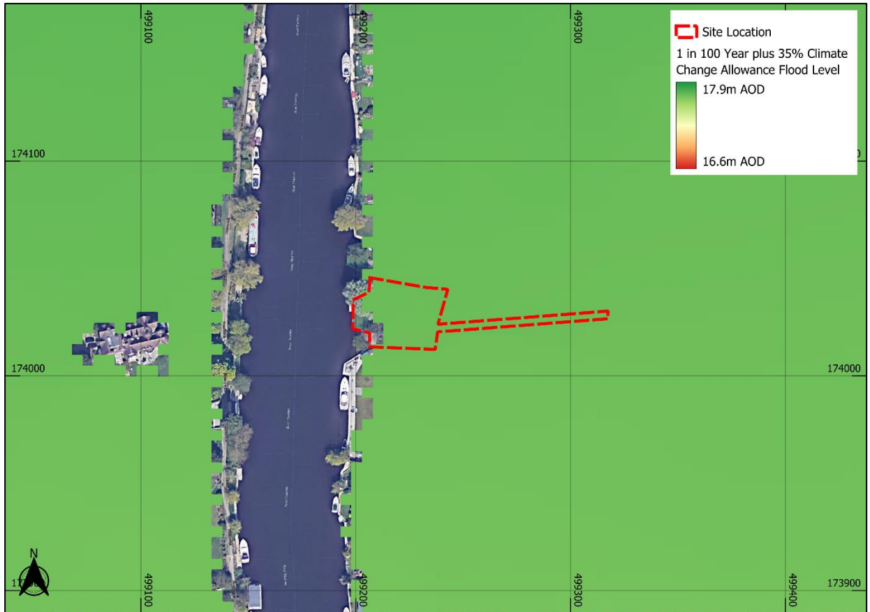
Figure 5: 1:100 year + climate change (35%) flood level (Base map from Google Hybrid © Contains public sector information licensed under the Open Government Licence v3.0)
