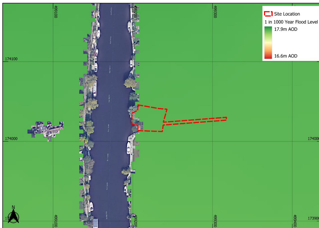
Figure 6: 1:1000 year flood level (Base map from Google Hybrid © Contains public sector information licensed under the Open Government Licence v3.0)
