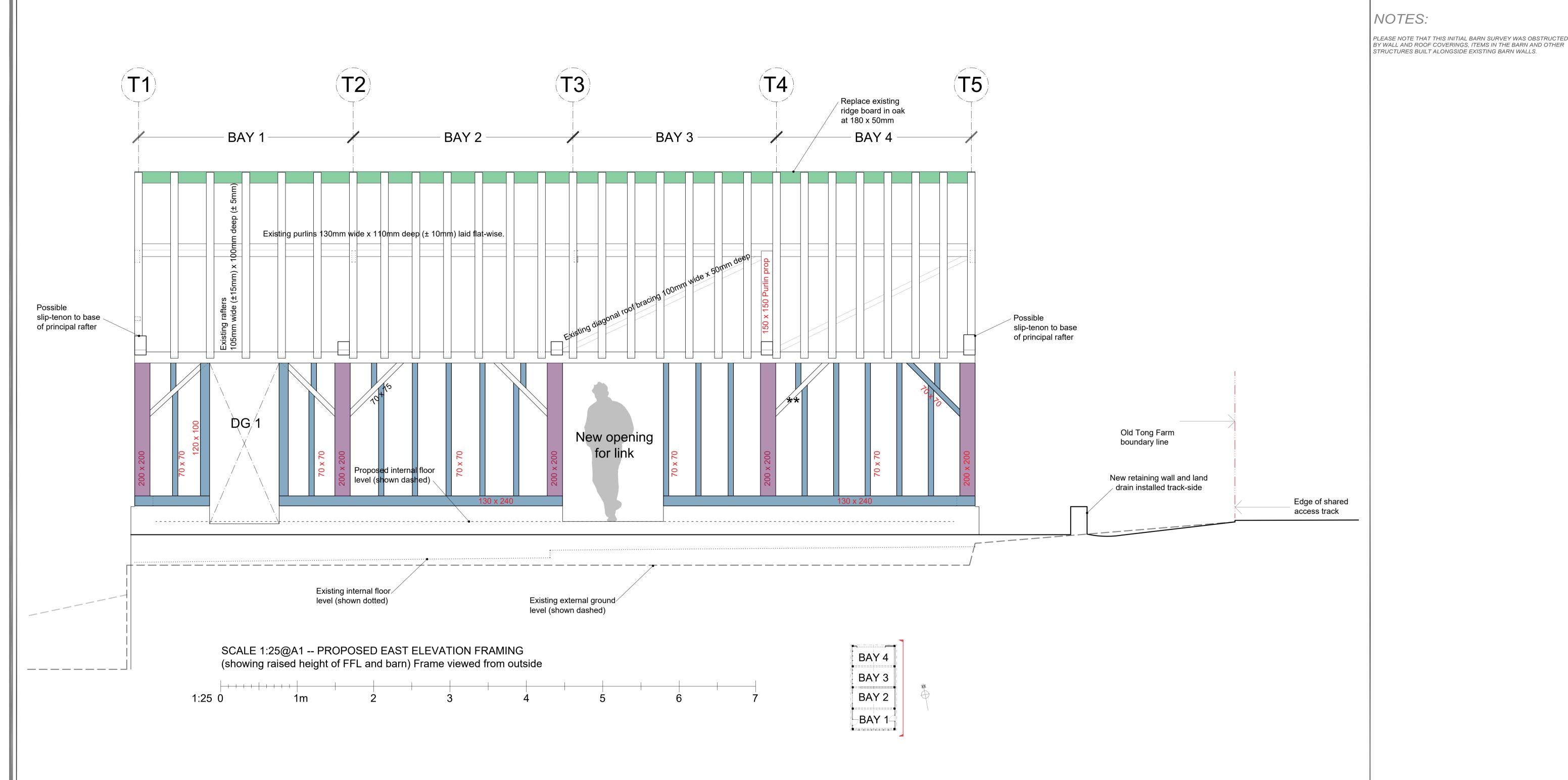
PLEASE NOTE!! INTERMEDIATE 'TRUSSES' ARE NOT TRUE TRUSSES AS THE RAFTER SET THAT HOLD THE COLLARS ARE COMMON RAFTERS THAT STEP TO THE SIDE OF THE TIE-BEAM.
