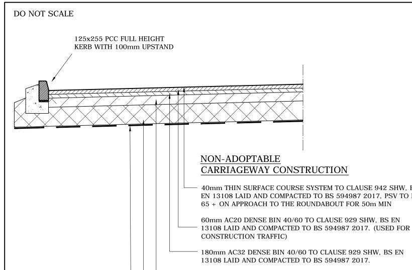
40mm THIN SURFACE COURSE SYSTEM TO CLAUSE 942 SHW, BS EN 13108 LAID AND COMPACTED TO BS 594987 2017, PSV TO BE
