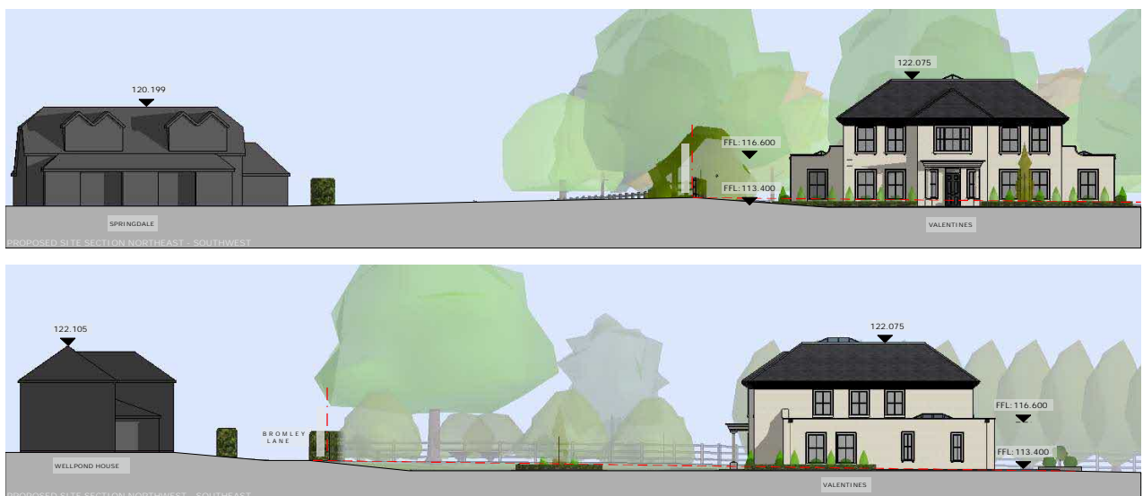
Figure 13: Section drawings showing the proposed house in relation to its neighbour to the east, Springdale, and the house to the north, facing it across the road, Wellpond House (extracts from drawing 340_PL15)
