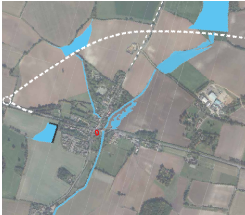
Figure 4: Reduction of flood risk due to Engineering works related to the Bypass. The site is now classed as being at very low risk (Figure 5)
