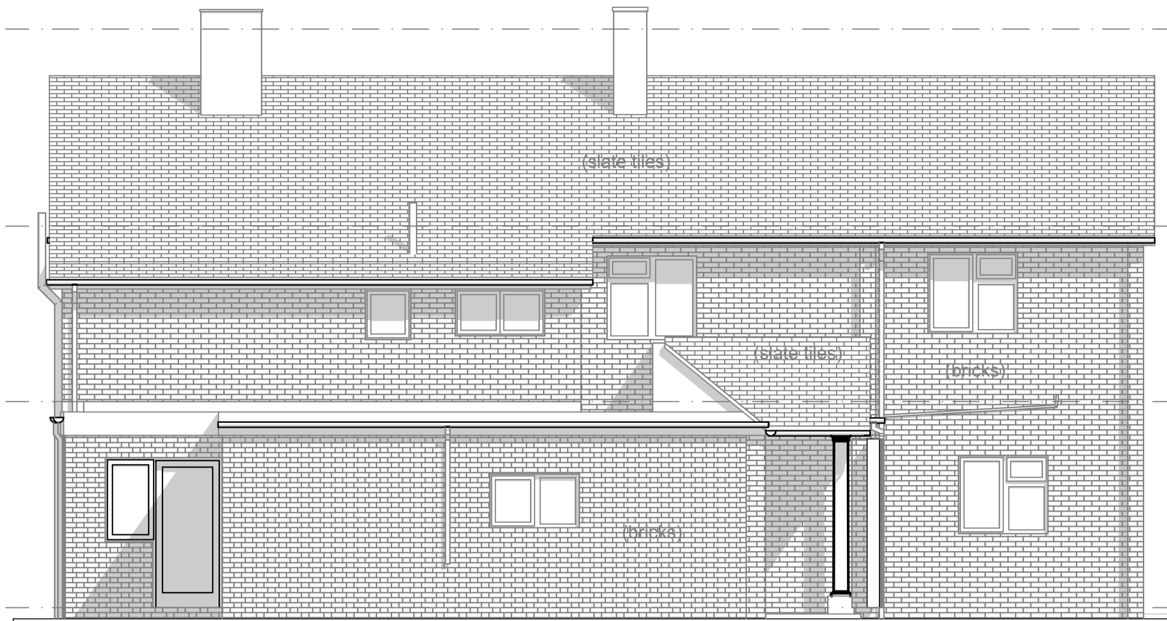
North Elevation - Existing 1:100
