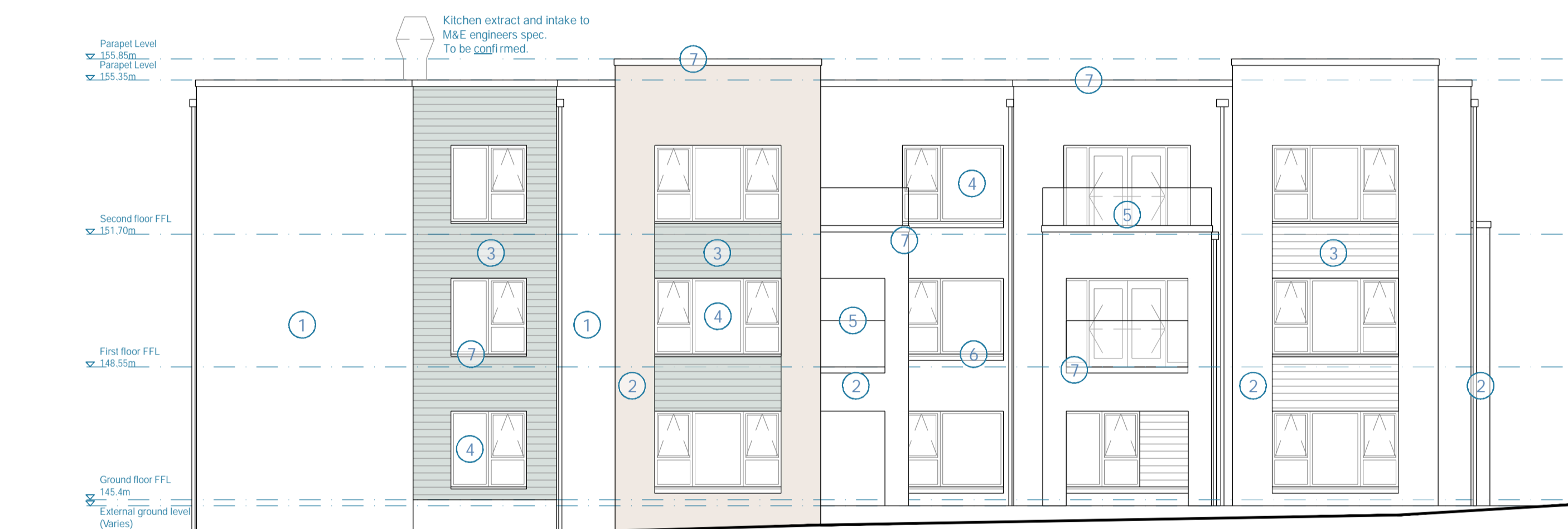
ELEVATION A: North-West Elevation (Left Elevation) Scale- 1:100
