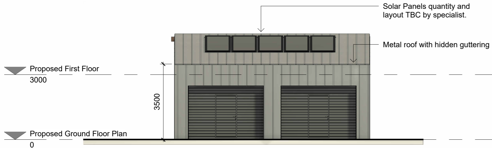
South Elevation - Garage 1 : 100
