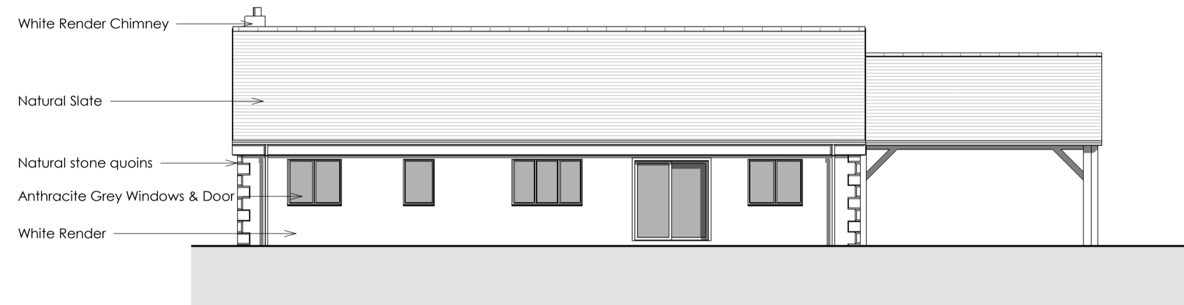
3 South West Elevation 1 : 100
