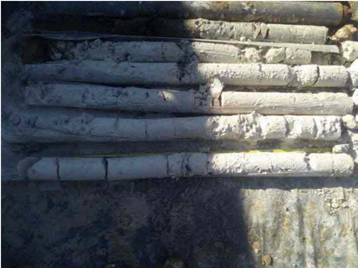
Photograph 2: BH01 encountered ground from 16.2mbgl to 25.2mbgl
