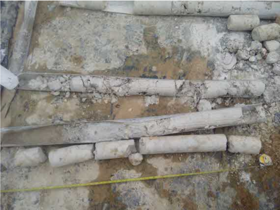
Photograph 5: BH01 encountered ground from 29.7mbgl to 35.7mbgl
