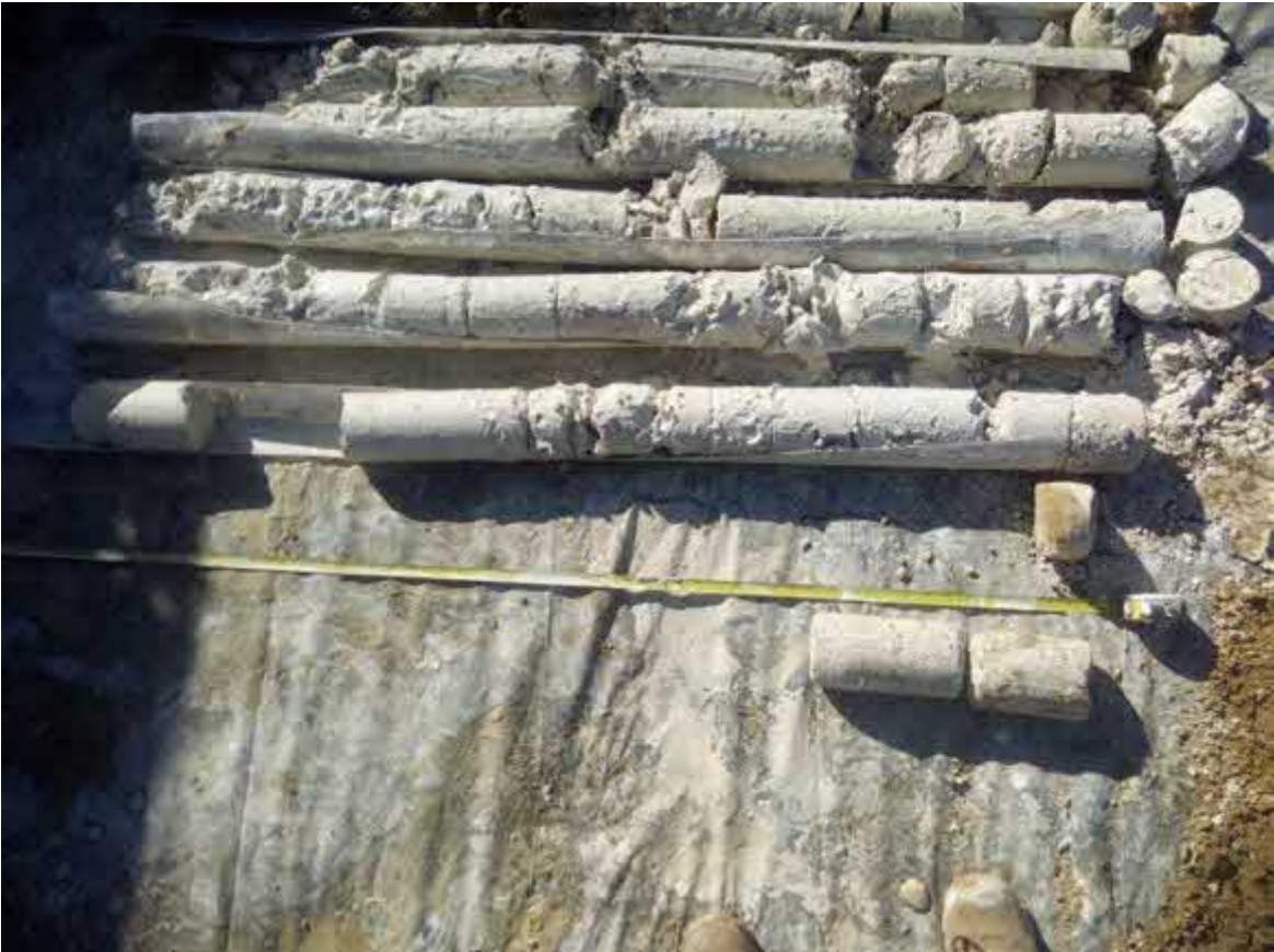
Photograph 3: BH01 encountered ground from 17.7mbgl to 28.2mbgl
