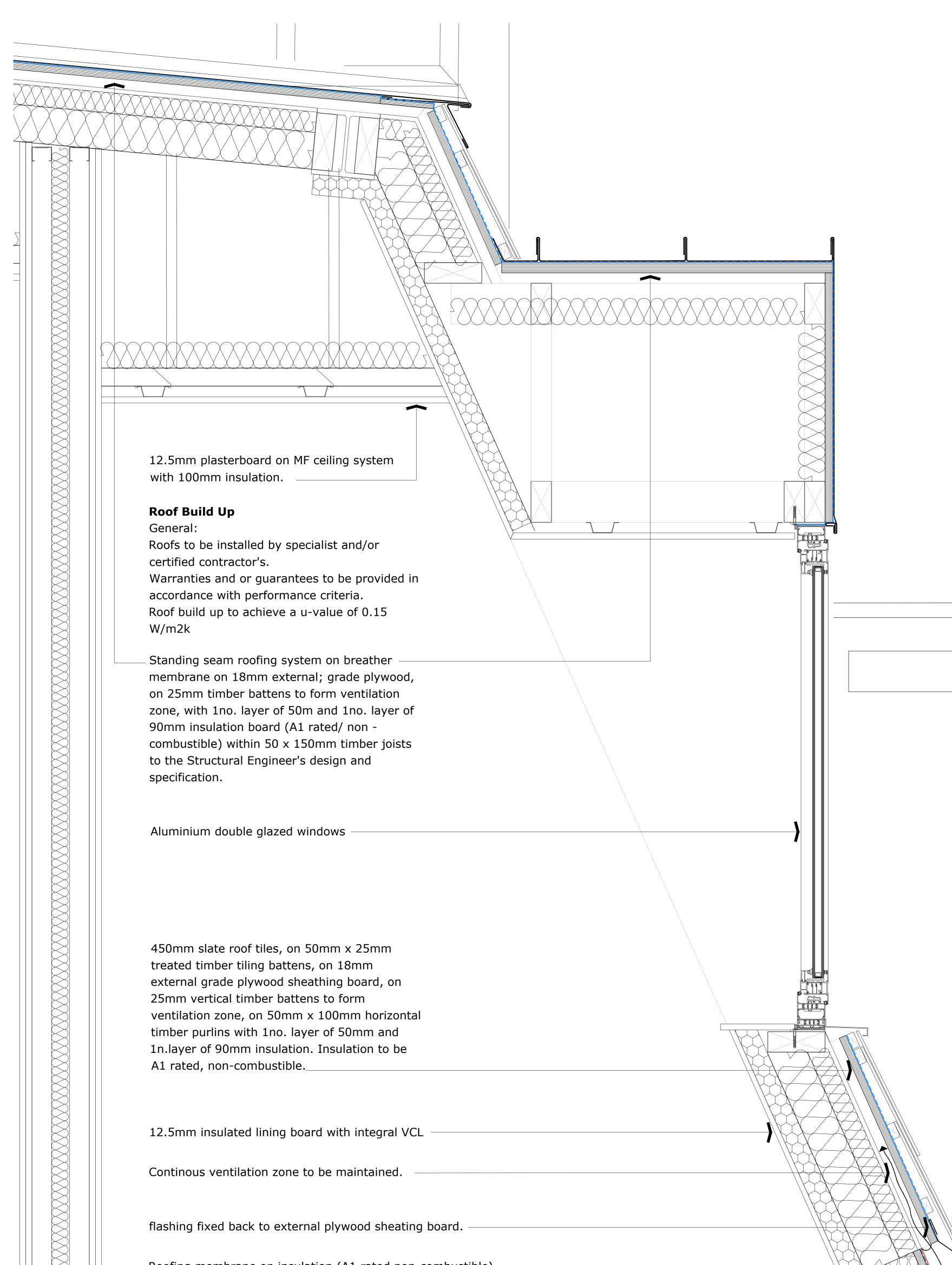
Standing seam roofing system on breather membrane on 18mm external; grade plywood, on 25mm timber battens to form ventilation zone, with 1no. layer of 50m and 1no. layer of 90mm insulation board (A1 rated/ non combustible) within 50 x 150mm timber joists to the Structural Engineer's design and specification.
