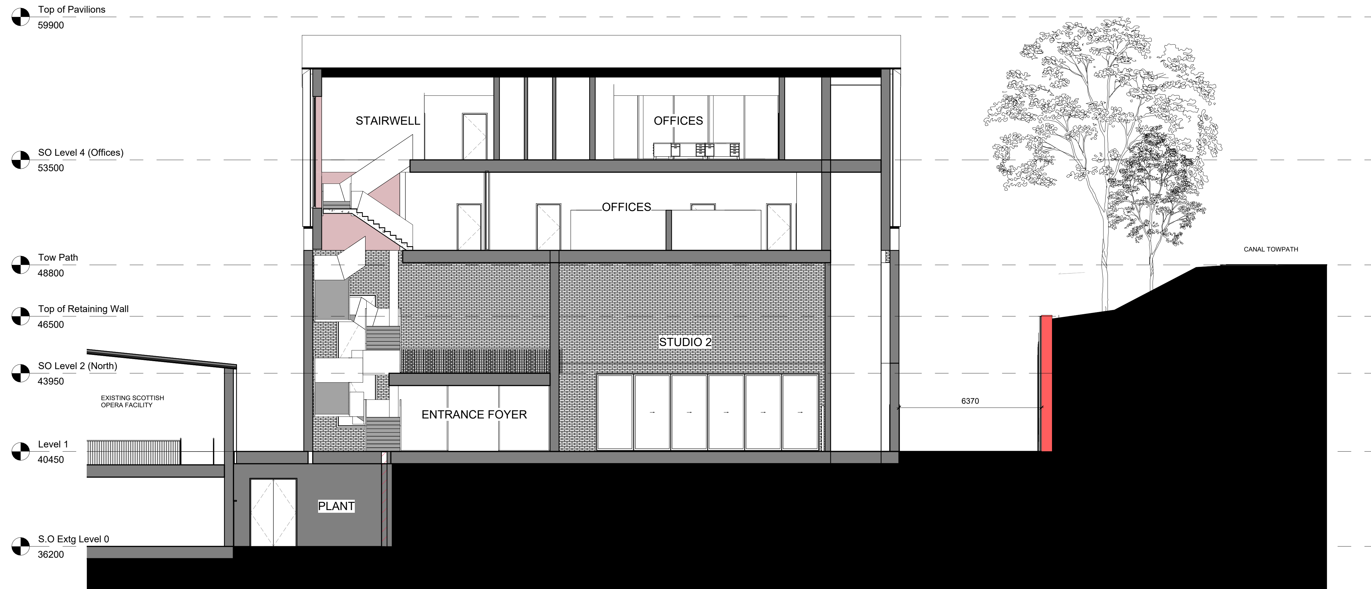
1 Scottish Opera cross section C-C (Office block) 1 : 100
