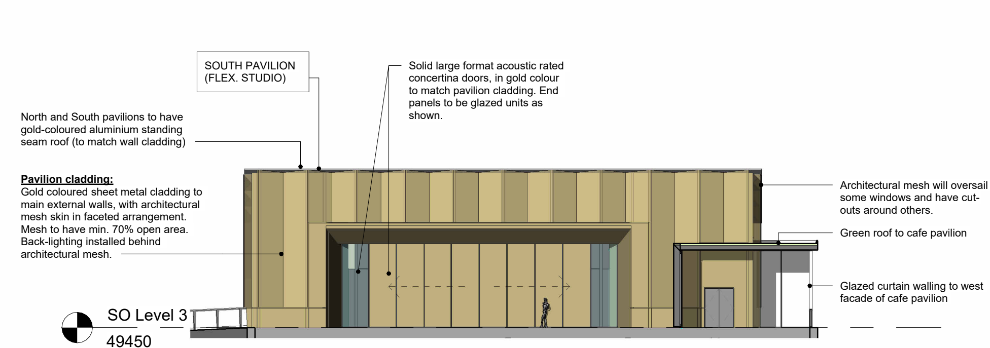
2 SO Elevation - Studio pavilion (North elev) 1 : 200
