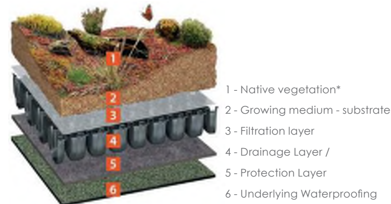
Figure 71 - Proposed buildup - Source: Bauder
