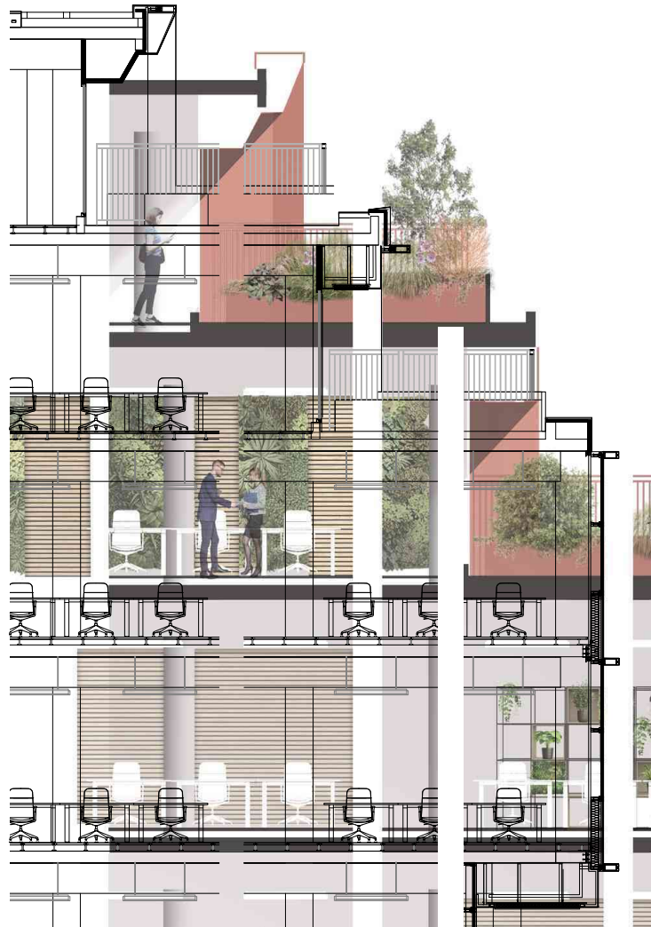
Proposed storey rod section - West facade
