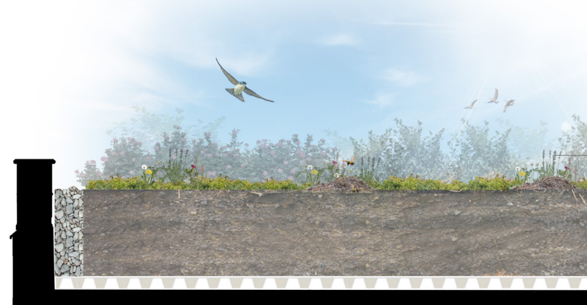
Figures 6- Green Roofs System - Source: Murray & Associates
