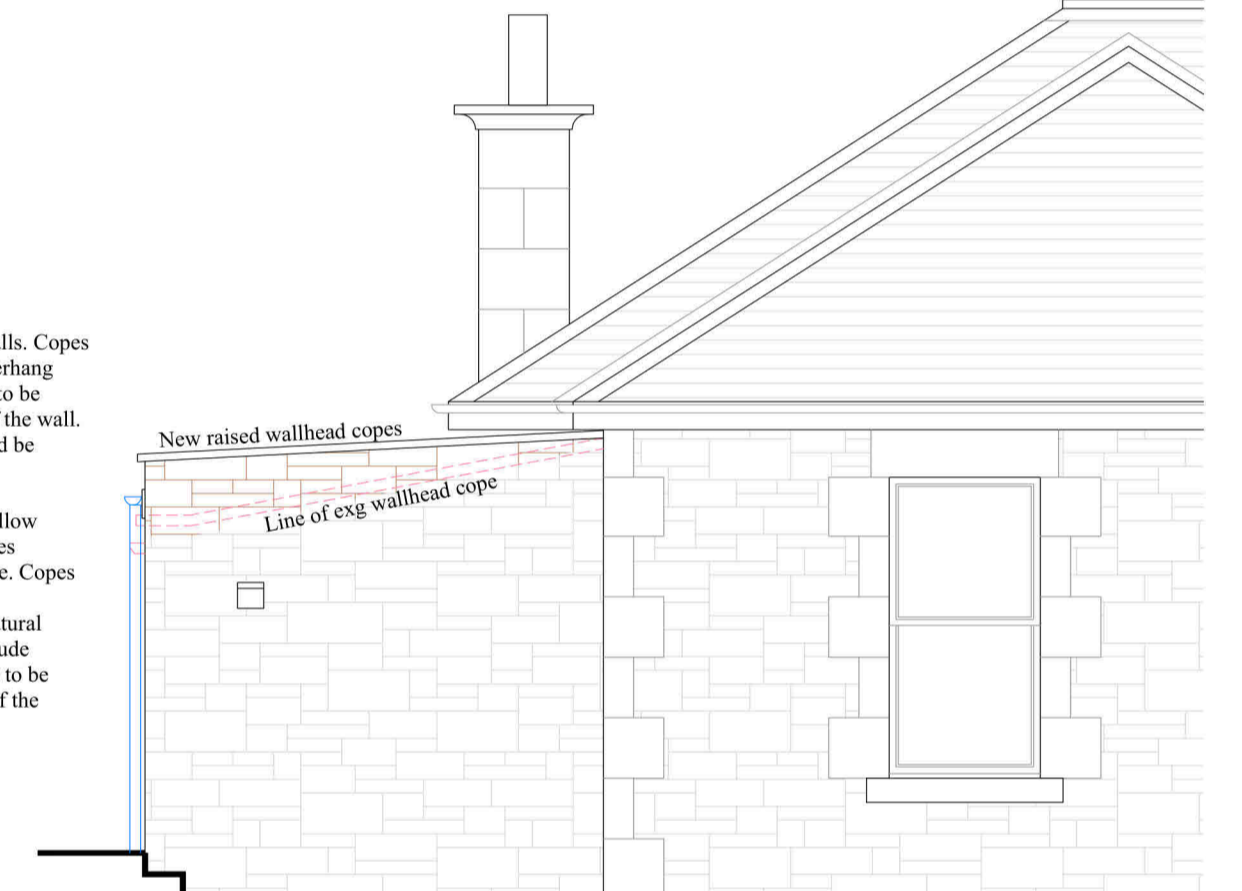
1:50 PART NORTH WEST ELEVATION AS PROPOSED
