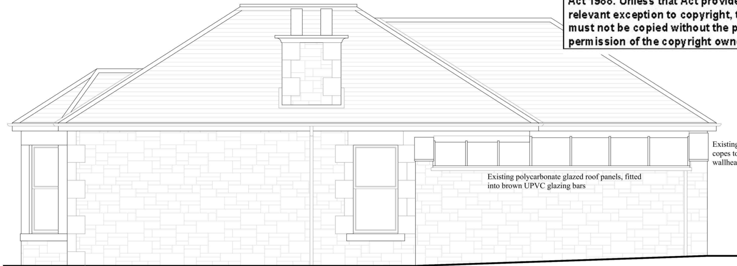
1:50 NORTH EAST ELEVATION AS EXISTING
