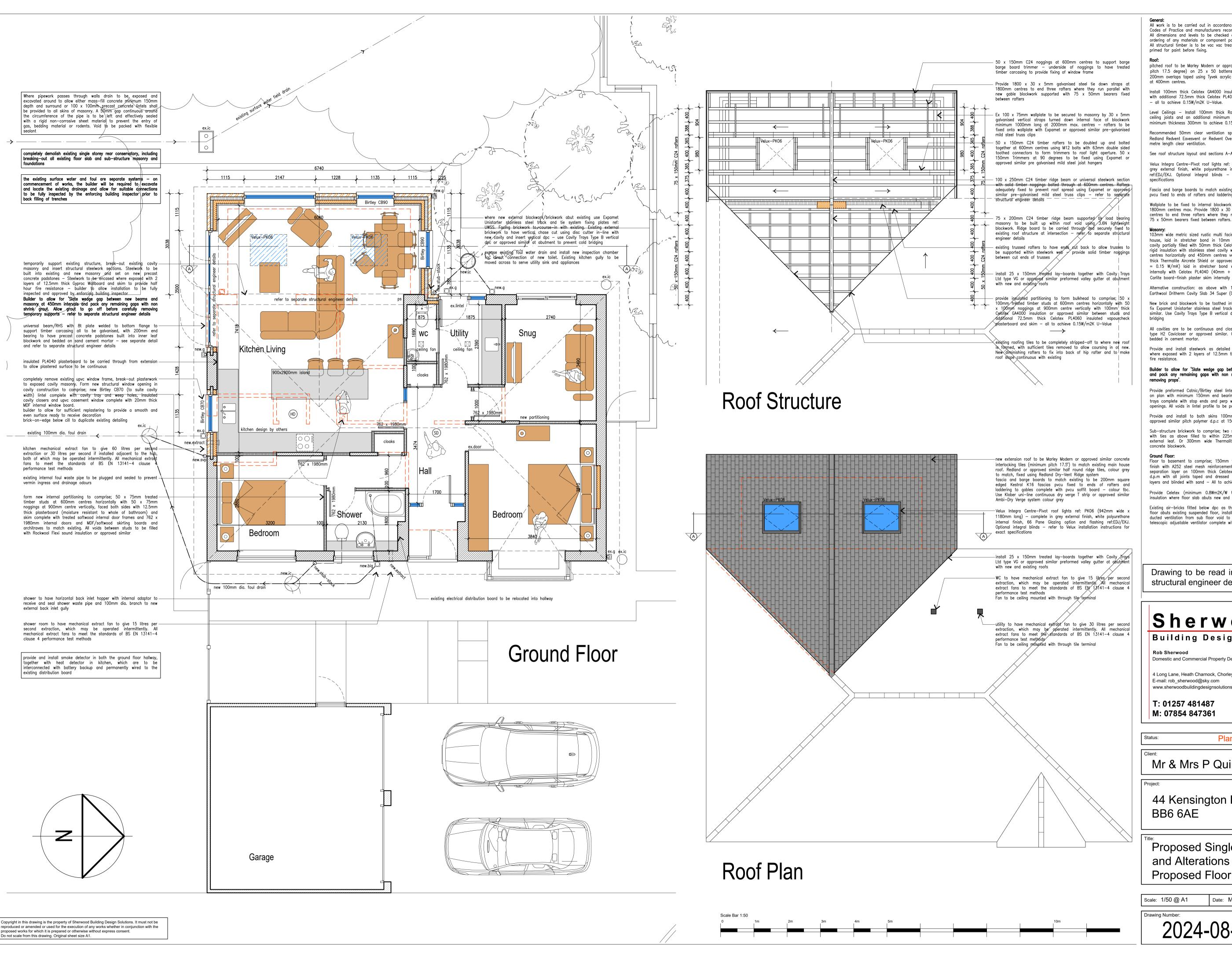
All work is to be carried out in accordance with local authority requirements. British Standards. Codes of Practice and manufacturers recommendations. All dimensions and levels to be checked on site prior to the commencement of work or the ordering of any materials or component parts. All structural timber is to be vac vac treated. All timber is softwood and is to be tanalised or
