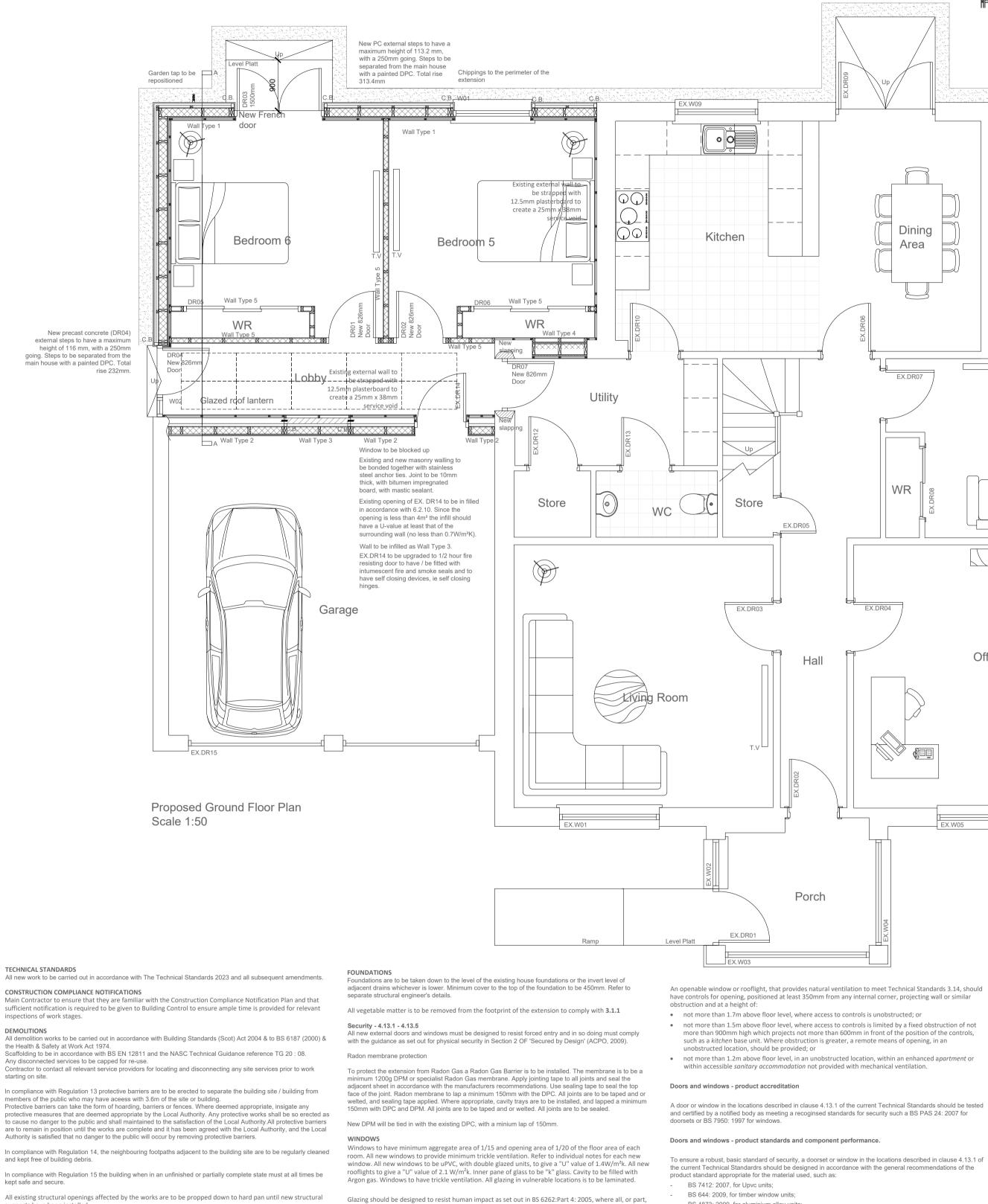
All existing structural openings affected by the works are to be propped down to hard pan until new structural supports have been installed.
