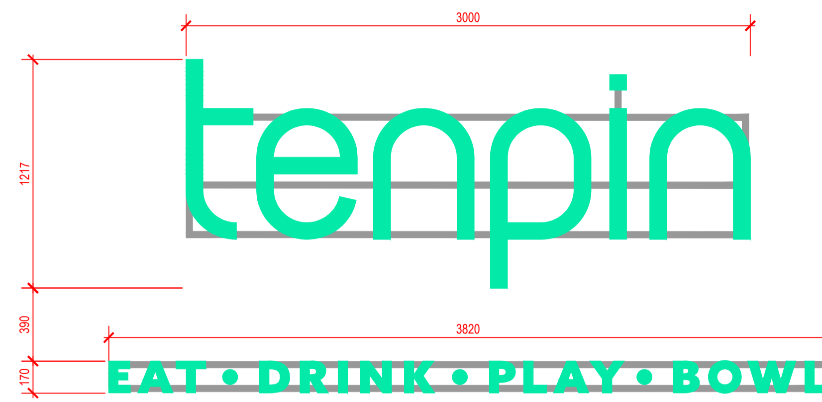
SIGN 01 SCALE 1:20 @ A1 3D Letters internally illuminated.
