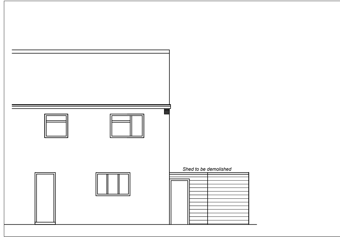
EXISTING REAR ELEVATION
