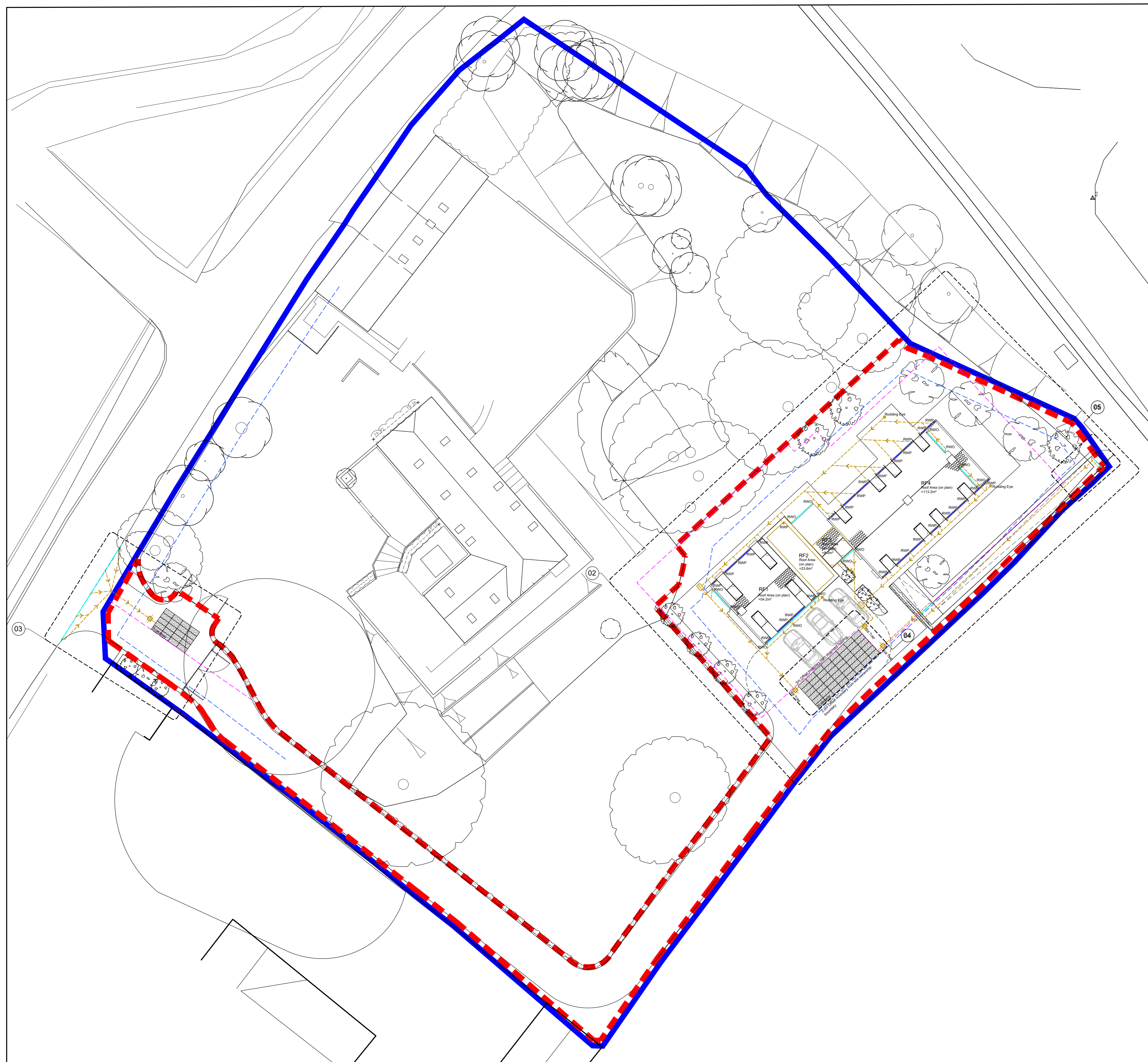
01 - Proposed Soakaway Locations (Scale 1:200 @ A0)
