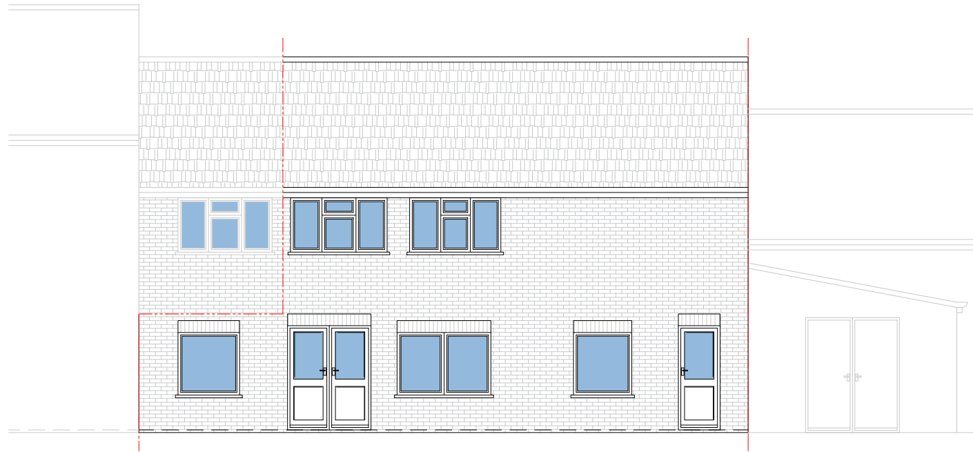
EXISTING FRONT ELEVATION 1:100
