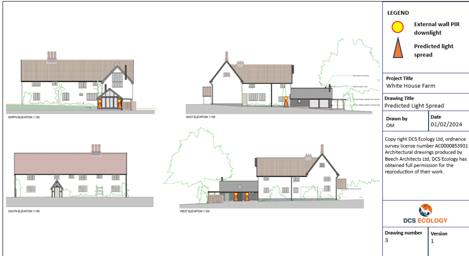
Figure 4: Placement of lighting on building exterior
