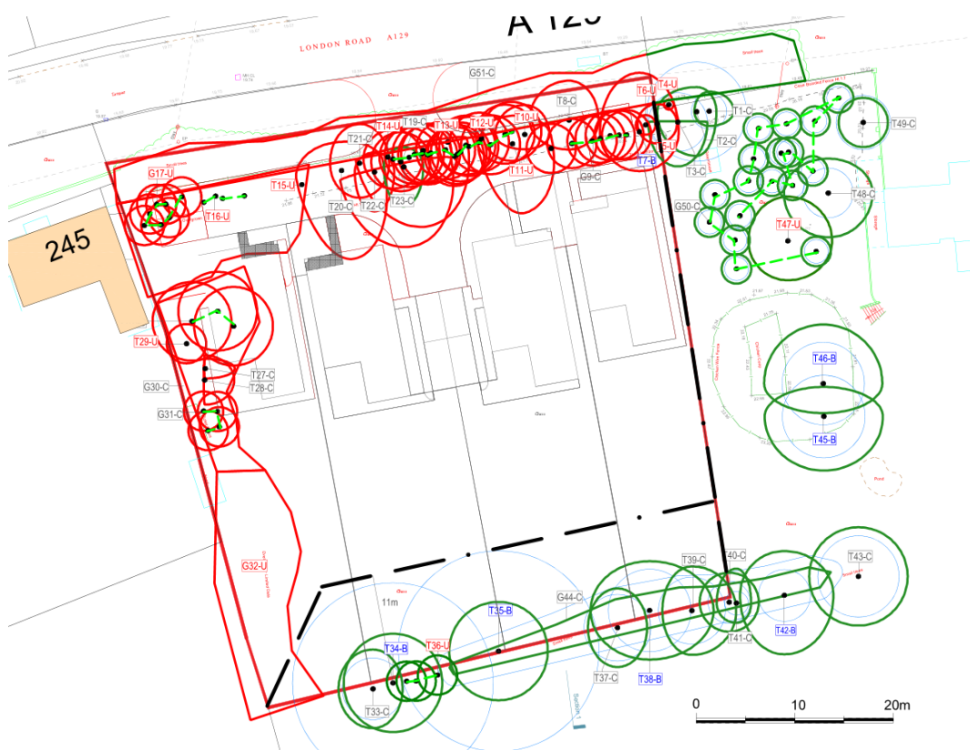
Plan 5 – extract from SHA 1776 TPP – do not scale, north is vertical. Green to be retained, red to be removed and black dashed lines – tree protection fencing.
