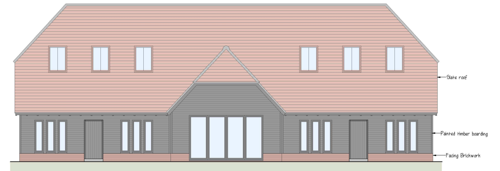
1: 100 Proposed Front Elevation Barn 2
