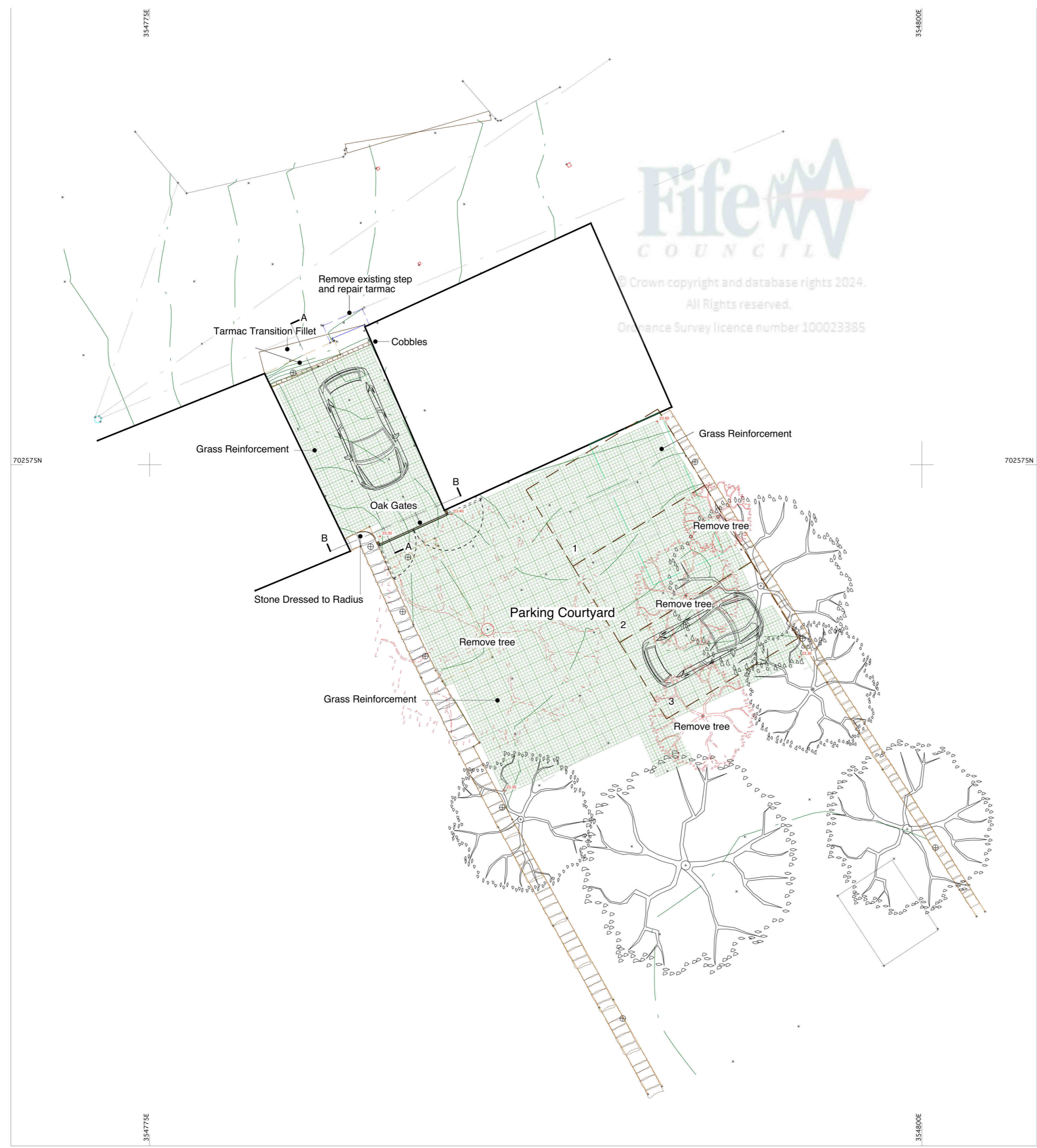
Grass Reinforcement Green Recycled High Density Polyethylene or equal and approved. Installed to manufacturers instructions.
