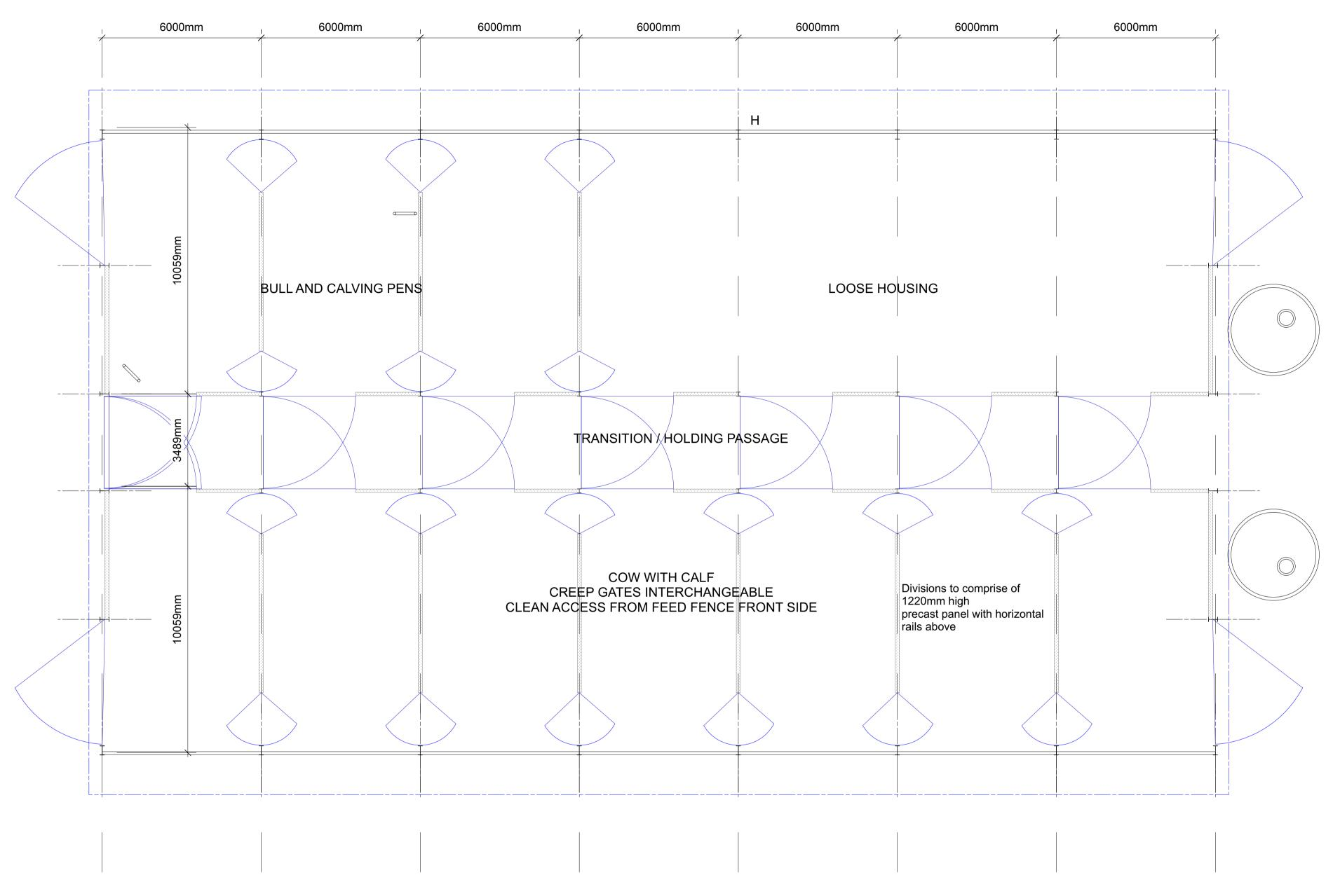
Gates and panels shown are indicative only and subject to change depending on pen sizes Mechanical ventilation system to be designed and confirmed in the next stages. HVLS (High volume low speed fans) with reverse funtion likely to be chosen)
