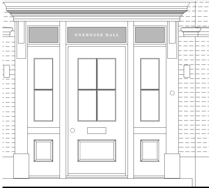
Figure 10. Elevation of Timber panelled front door with lights. Glazing shall be narrow double glazing with integral glazing bars. Over the door an acid-etch glazing panel 'Onehouse Hall' in clear glazed lettering.
