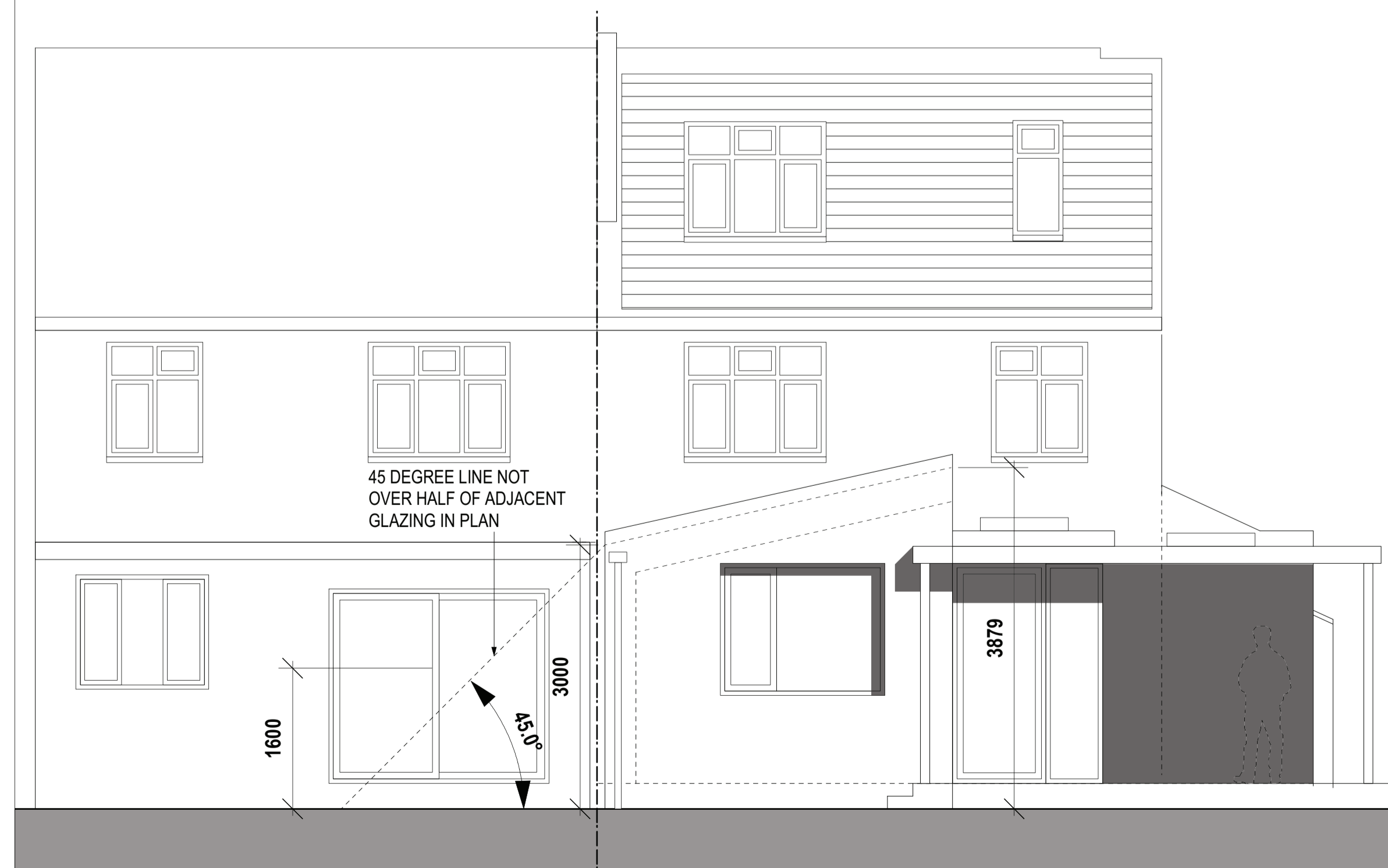
PROPOSED REAR (WEST) ELEVATION
