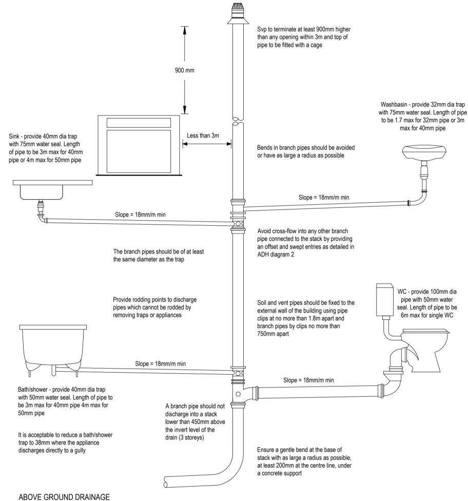
All new above ground drainage and plumbing to comply with BS EN 12056-2:2000 for sanitary pipework. All drainage to be in accordance with Part H of the Building Regulations. Wastes to have 75mm deep anti vac bottle traps and rodding eyes to be provided at changes of direction.
