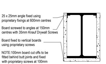
Supply and install new structural elements such as new beams, roof structure, floor structure, bearings, and padstones in accordance with the Structural Engineer's calculations and details. New steel beams to be encased in 12.5mm Gyproc FireLine board with staggered joints, Gyproc FireCase or painted in Nullifire S or similar intumescent paint to provide 1/2 hour fire resistance as agreed with Building Control. All fire protection to be installed as detailed by specialist manufacturer.
