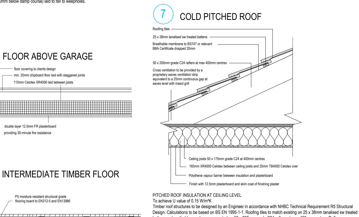
battens on breathable membrane supported on 50 x 200mm grade C24 rafters at max 400mm centres. Rafters supported on 100 x 50mm sw wall plates. Insulation at ceiling level to be 165mm XR4000 Celotex between ceiling joists with a further 25mm TB4000 Celotex over joists.
