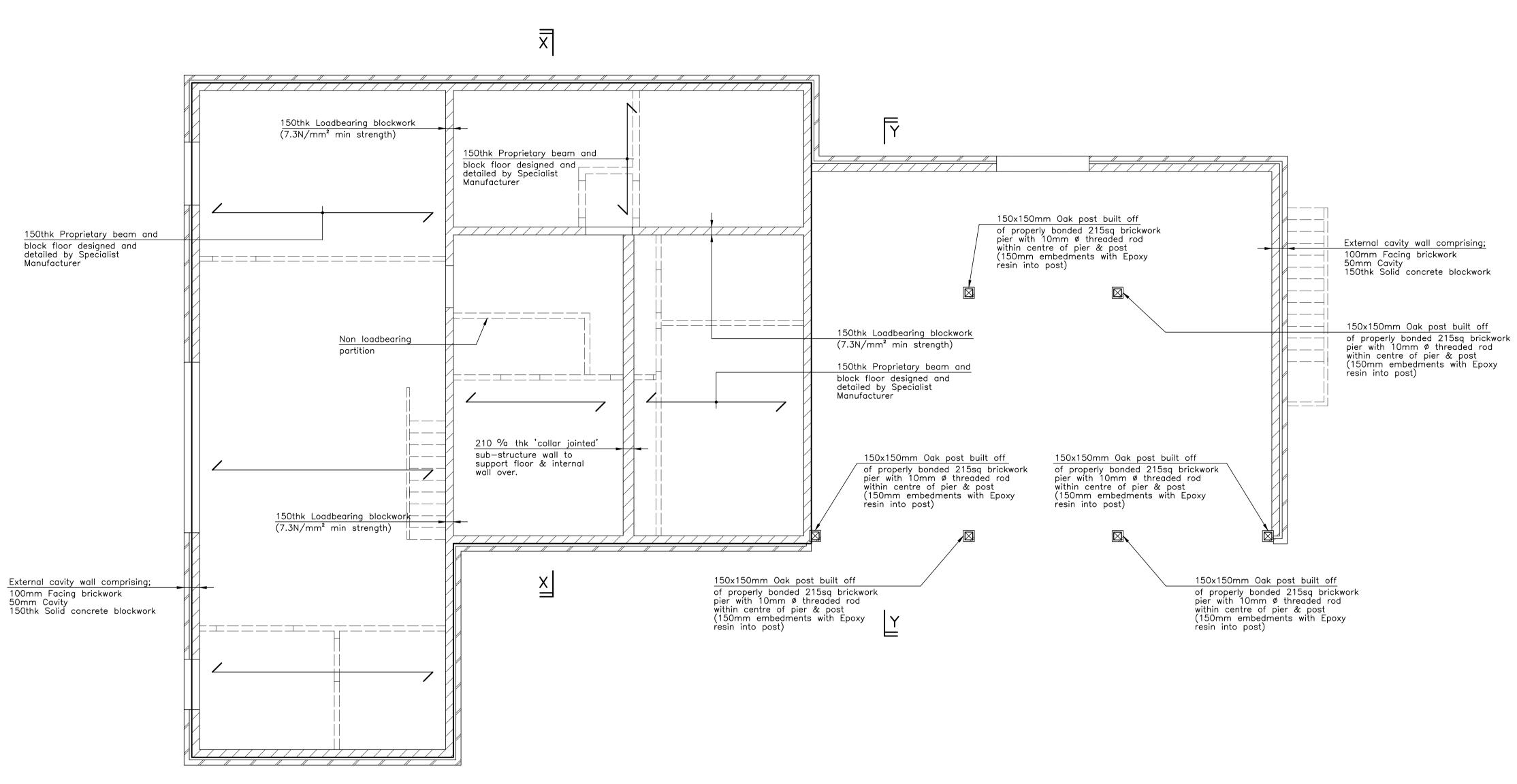
PLAN AT GROUND FLOOR LEVEL SHOWING SUPPORTING CONSTRUCTION IN FULL Ground floor to be 150mm thk proprietary pre-cast concrete beam and infill block floor designed and supplied by Specialist Manufacturer. Span direction thus on plan:
