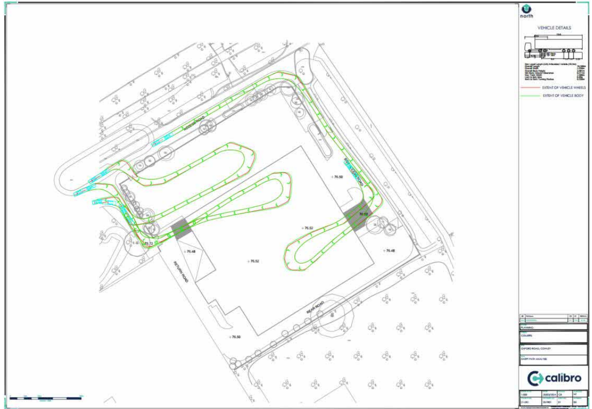
Figure 3-1 Swept Path Analysis– 16.5m Articulated Vehicle
