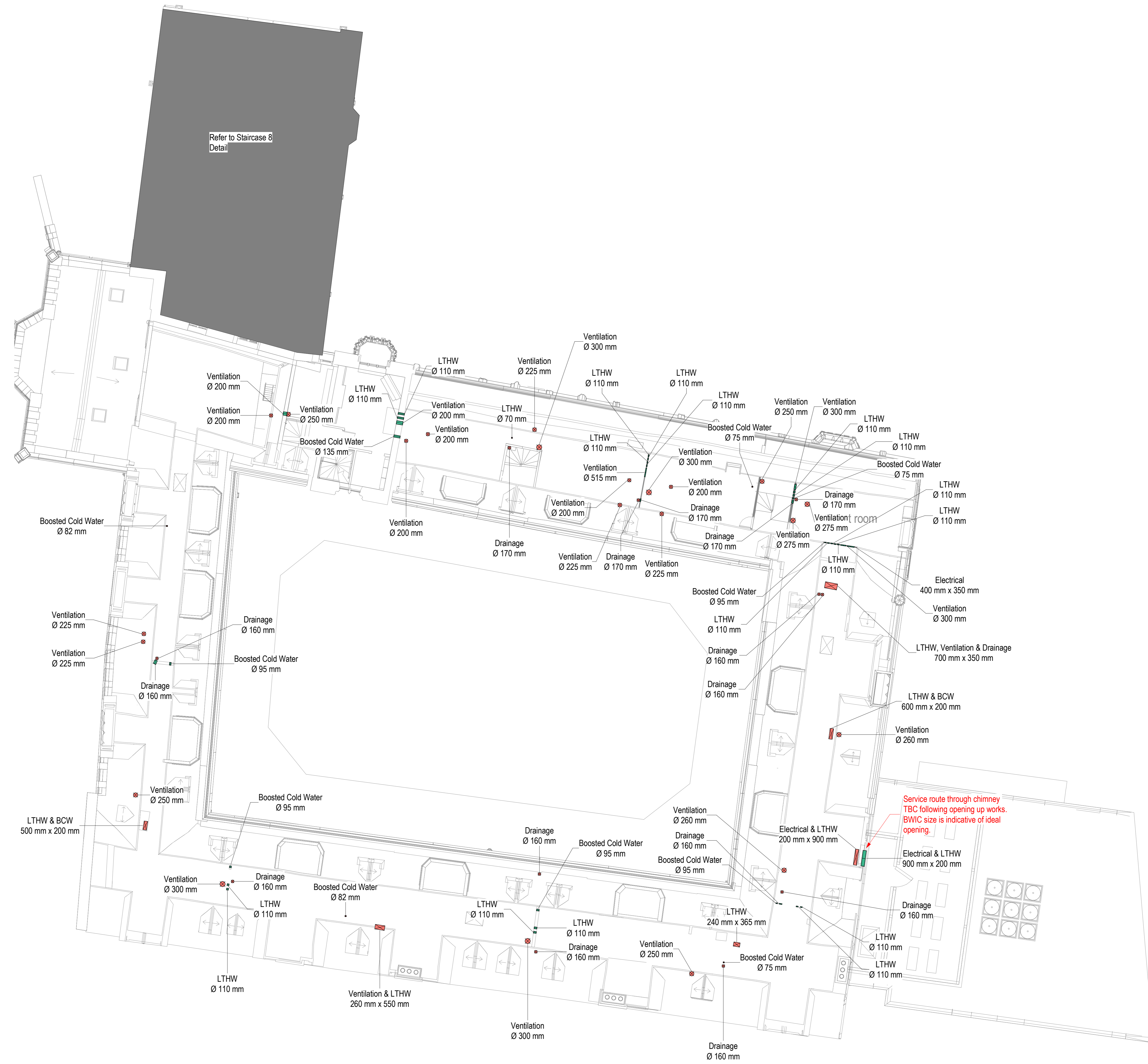
1 500 - Builders Work in Connection - Loft (Old Quad) 1 : 100
