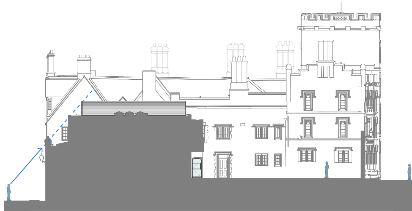
Elevation E01 – Proposed east elevation of Old Quad, showing no sightline from street level to ASHP enclosure
