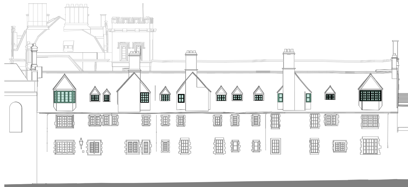
South elevation of Old Quad, facing Brewer Street; windows to be replaced are highlighted in green
