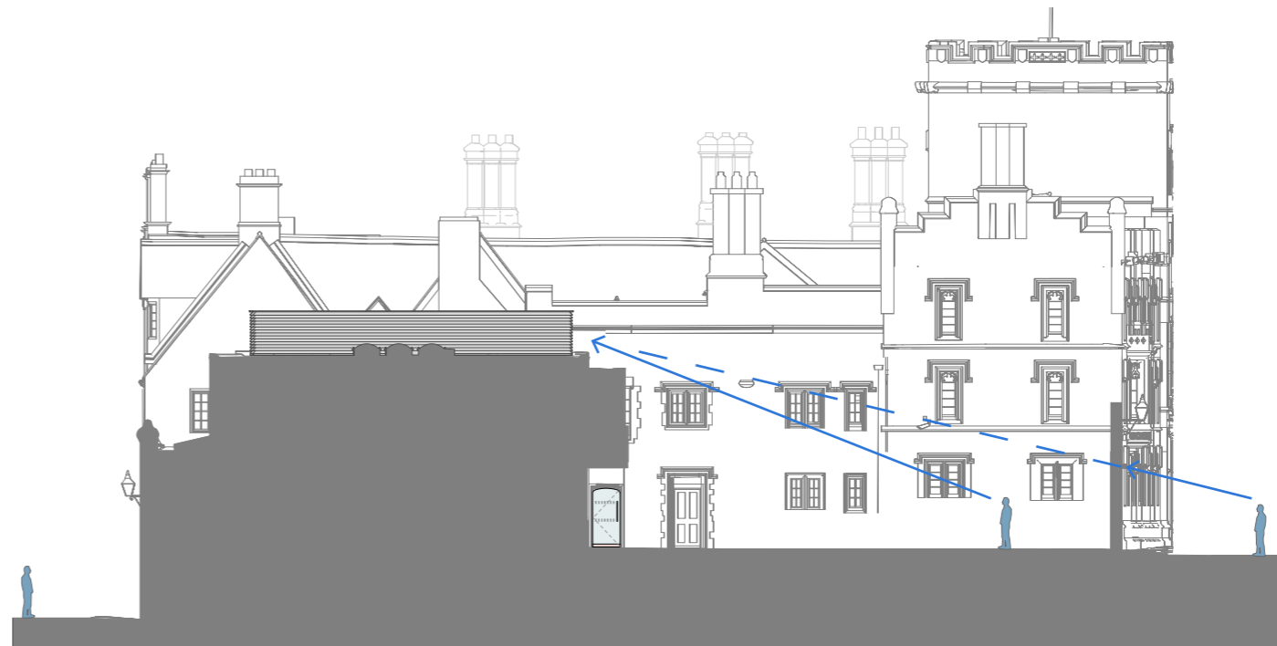
Elevation E01 – Proposed east elevation of Old Quad, showing sightlines from Pembroke Street and Library Court
