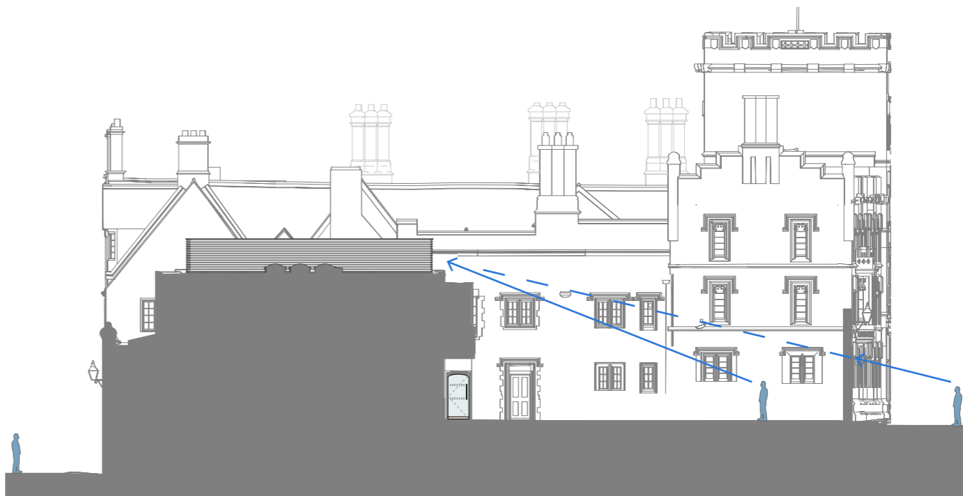
Elevation E01 - Proposed east elevation of Old Quad, showing sightlines from Pembroke Street and Library Court
