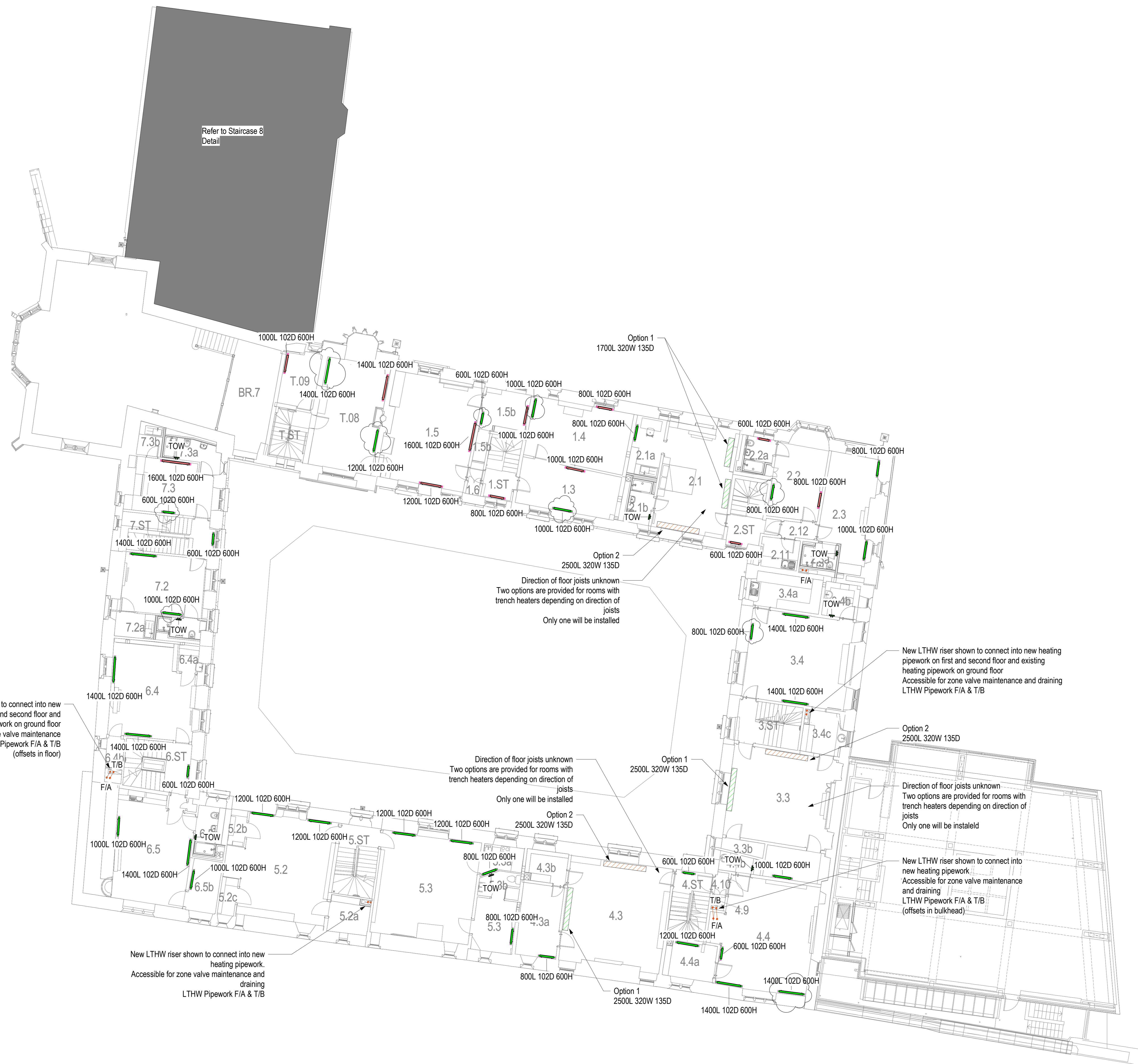
500 - Heating (Detail) - Level 01 - Old Quad 1 : 100
