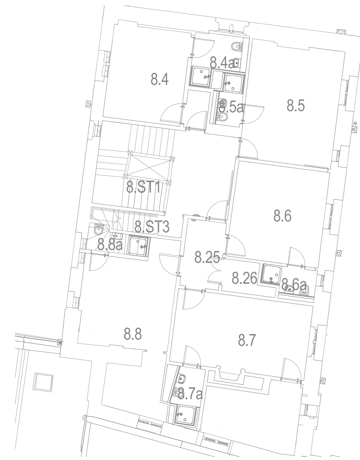
2 500 - Builders Work in Connection - Level 02 (Staircase 8) 1 : 100
