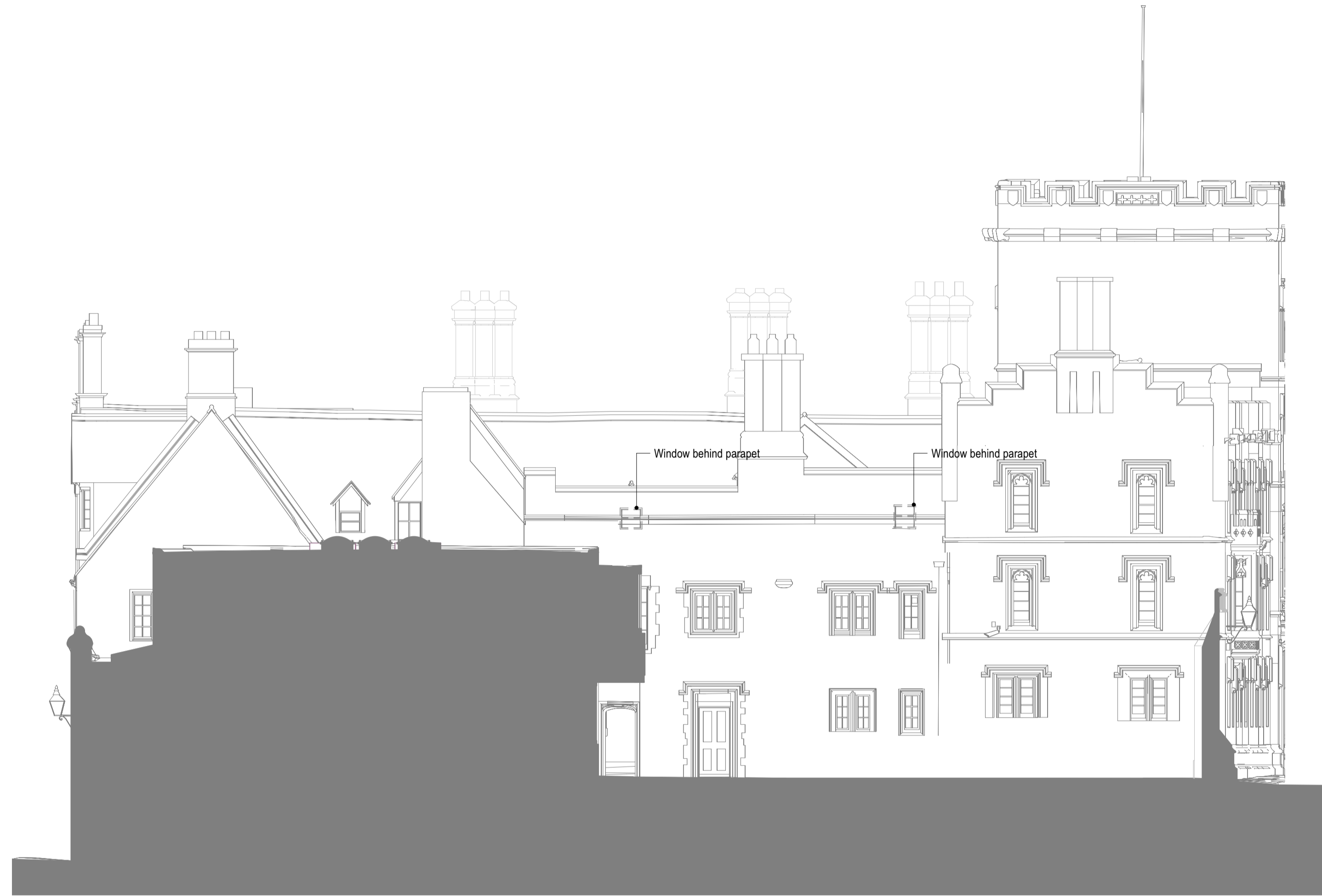
Elevation 05 Old Quad east elevation 1:100@A1
