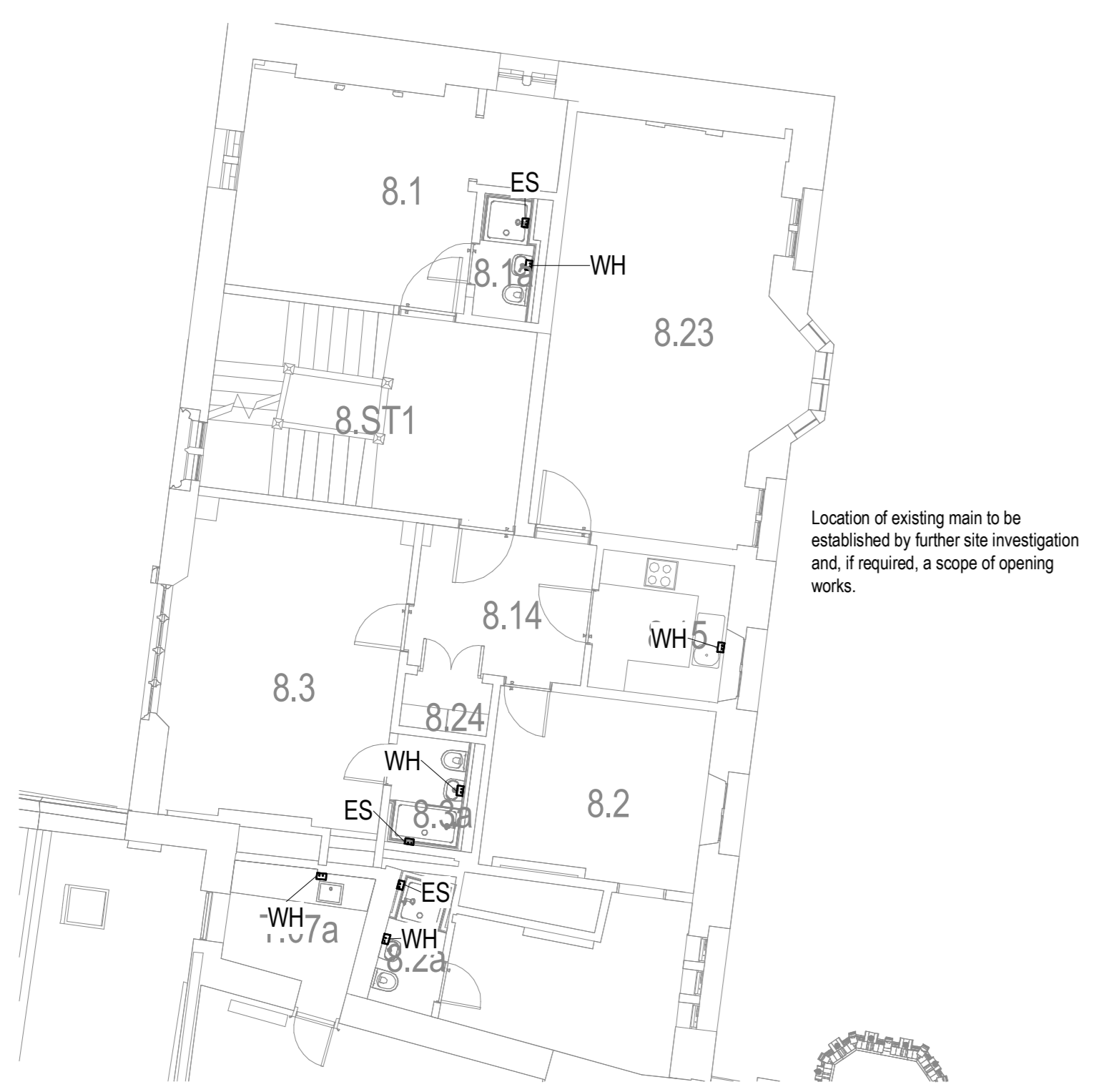
2 500 - Piped Supply (Detail) - Level 01 (Staircase 8) - Staircase 8 1 : 100
