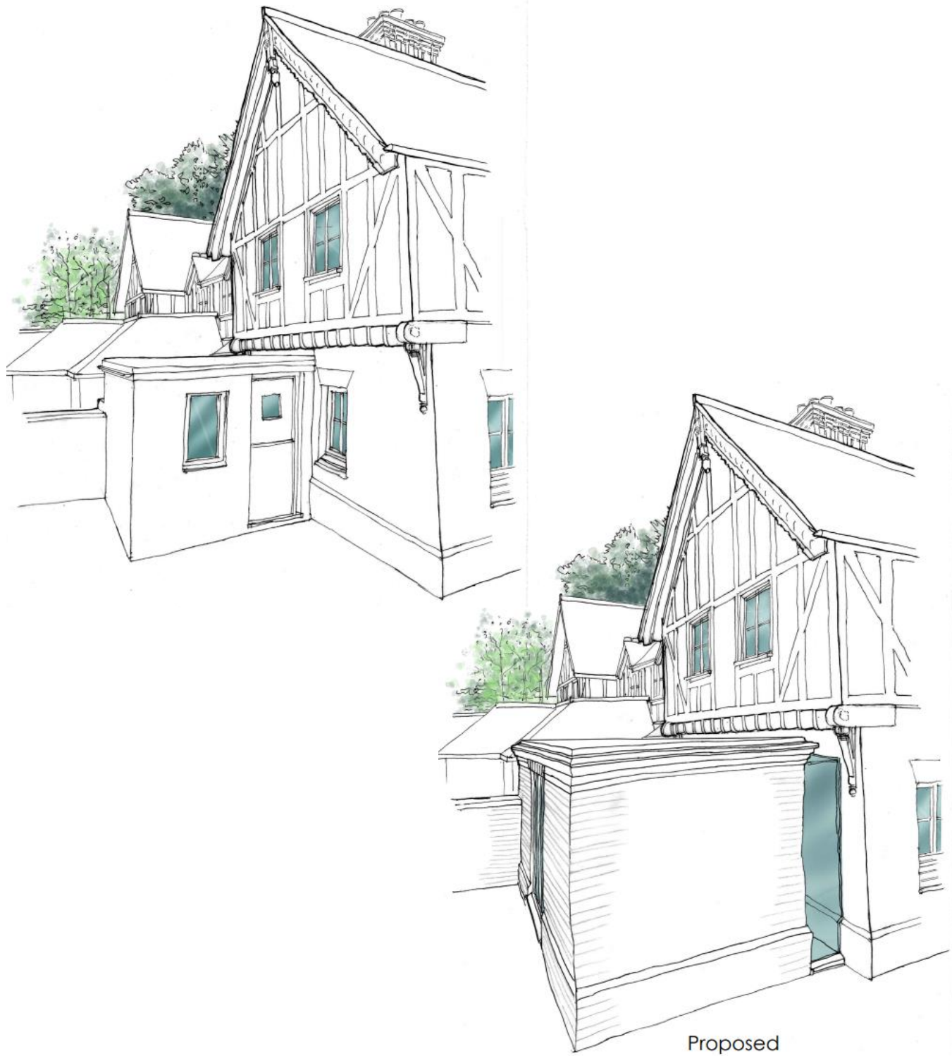
Figure 14: Illustration of rear of Fielders with existing extension (left) and proposed extension (right)
