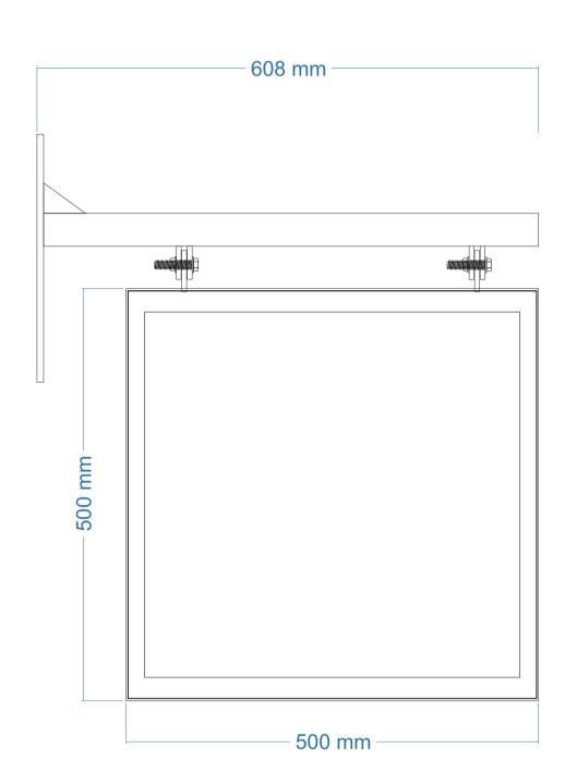
steel internal frame and wall bracket epc black with 3mm folded ACP face trays finished semi matt grey RAL 7016.
