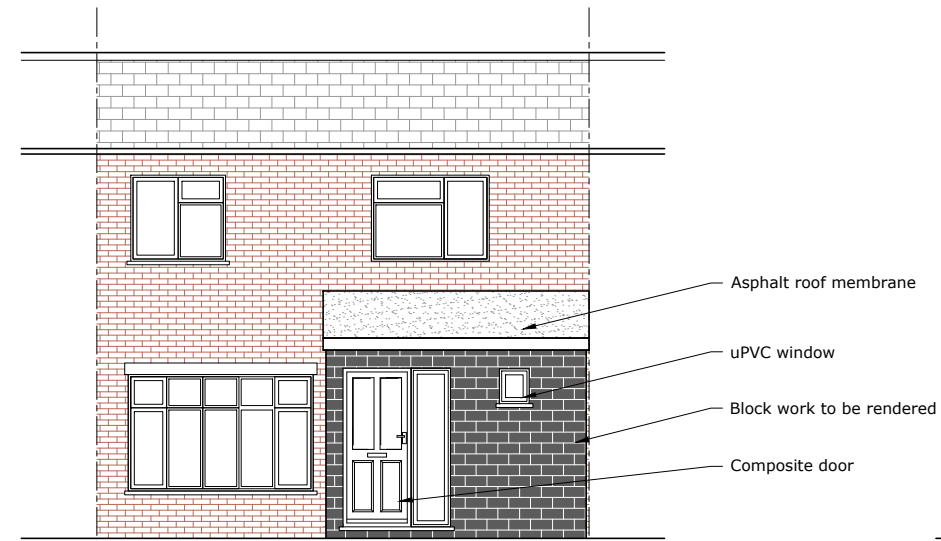
EXISTING LEFT ELEVATION SCALE 1:100 0 1 2 3 4 5m
