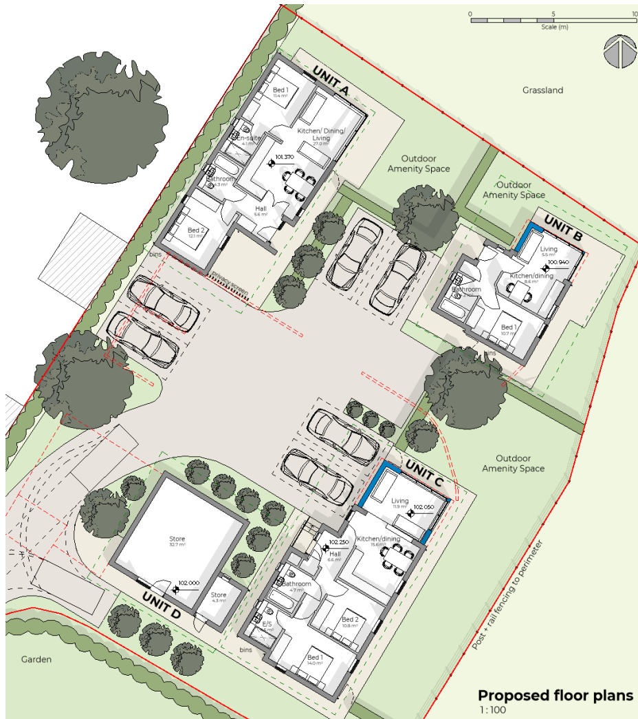
Figure 3 Proposed site layout showing extensions to Units B & C highlighted with blue infill walls
