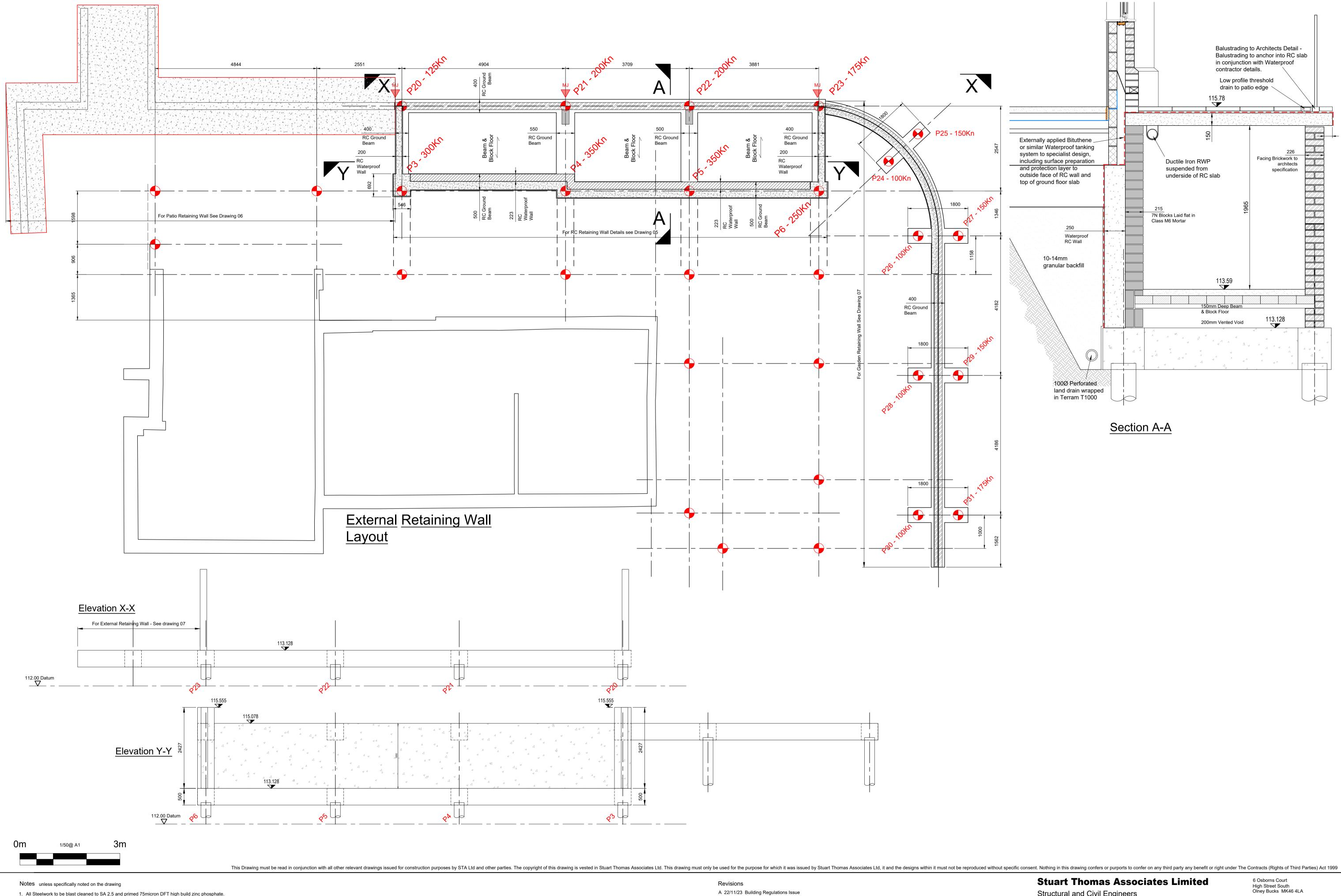
All Steelwork to be blast cleaned to SA 2.5 and primed 75micron DFT high build zinc phosphate. Steelwork to be designed fabricated erected in accordance with NSS and BS 5950.
