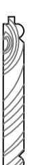
SECTION DETAIL THROUGH THE RIGHT HAND GATE BOARD OF EACH GATE (WHEN VIEWED FROM MARKET PLACE) SCALE: 1:5
