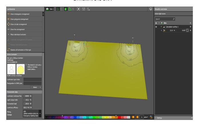
The above imaging is the output results from an industry standard lighting calculation program called DIALux. It shows the location of the 2 no lighting columns on the far side of the car park of the nursery building. As can be seen from the output illustration above the illumination level is quite high directly under the location of each column and fades off towards the end of the car park.
